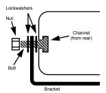
**SC-1012 Remote Panel:** The remote panel of the SC-1012 is typically mounted underneath the vehicle dashboard using mounting hardware (not supplied). Mount the panel in a location away from the driver's or passenger's legs.
